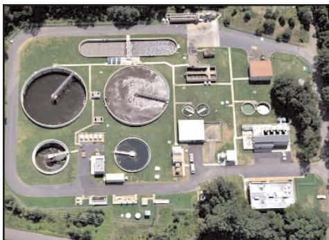
The Remington Plant can treat up to two million gallons of sewage per day.
